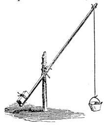
from 4 to 12 feet. The bucket may be made of canvas, basket-work, leather, wood, or almost any other material; leakage, though considerable, is of little consequence, because the action of the apparatus is so quick, that there is not time for much water to be lost. This contrivance is used over almost the whole globe-less in England than elsewhere; it is very common where long poles can
