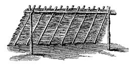
for flooring above the snow or damp. A common plan is to support a cross-bar by two uprights, as shown in the figure; against this cross-bar a number of poles are made to lean; on the back of the poles abundance of fir branches are laid horizontally; and lastly, on the back of these are another set of leaning poles, in order to secure them by their weight.
