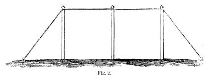
each end (fig. 2). Two sheets, A and B, are buttoned together and thrown over the cord, and then two other sheets, c and D; and c is buttoned to A, and D to B (fig. 3). Lastly another sheet is thrown over each of the slanting cords, the one buttoned to A and B, and the other to c and D; and thus a sort of dog-kennel is formed, in which six men-the bearers of the six pieces of canvas-sleep. The sides of the tent are of course pegged to the ground. There are many modifications
