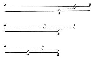
Let A o be the log. Cut two notches (1), (2), on opposite sides. Hold the log by the end A, and strike the end violently against the ground; the piece o, 1, 2, will fly off. Then make the cut (3) on the side opposite to (2), and again strike, and the piece 1, 2, 3, will fly off. So again with cut (4), &c. (Peal.)
