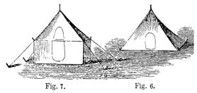
though by taking an additional joint to the tent-pole, and using tent-ropes (as may also be done with any other kind of tent), it may be made more airy by being raised up, and by having walls added to it (fig. 7). In default of canvas, the walls may be constructed of other materials. (See "Materials for Huts.")
