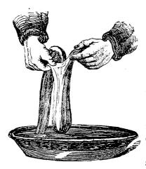
out, which is easily to be done by turning a very short piece of it inside out, just as you would turn up the cuff of your sleeve; then, catching hold of the turned-up cuff, dip the whole into a bucket, and scoop up a little water between the cuff and the rest of the gut. The weight of this water will do what is wanted : it will bear down an additional length of previously unturned gut; and thus, by a few succes-
