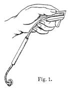
wick, a roll of touch-paper, a mass of hair of certain plants, and a long string of pith sewed up in a sheath. To ignite these, we must hold them as in fig. 1, and use the steel to strike downwards upon the flint. In the second division (b) are:—tinder of burnt rags, tinder of any kind with grains of gunpowder strewed over it, and touch-wood. All these require tinder-boxes, as explained below. There are also many other
