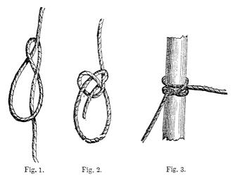
tight. The stick will enable you, at will, to untie the knot to break its back, as the sailors say—with little difficulty. A bowline is firmer, if doubled; that is, if the free end of the cord be made to wrap round a second time.
