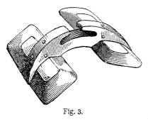
ther, as in figs. 1 and 2, using raw hide in addition to nails or pegs. Stuffed cushions must be secured inside the planks by tying or otherwise. With a saw and a mortise-chisel, a saddle of the pattern shown in fig. 3 would be easy to make. It is stronger than the one just described, and
