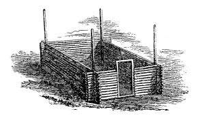
spaces between the logs must be caulked with moss, &c., or the log-cabin will be little better than a log-cage. It requires a great many logs to make a hut; for, supposing the walls to be 8 feet high, and the trees to average 8 inches in diameter, twelve trees would be required to build up one side, or fortyeight for all four walls. Other timber would also be wanted for the roof.
