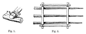
The raft-fastening in common use, is shown in fig. 1 : it is a stout, lithe wand, bent over the cross piece, and wedged into holes in the framework.
