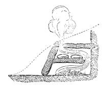
and two flat stones are slid horizontally, like shelves, into grooves made in the sides of the hole, as shown in the figure; where it will be observed that the uppermost stone does not quite reach to the face of the bank, and that the lowermost stone does not quite reach to the back of the \*
