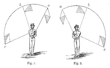
The signalman may work from left to right, or from right to left, as shown in figs. 1 and 2, according to convenience and the direction of the wind. To make a short flash, the flag is waved from a to b, and back to the normal position a. To make a long flash, the flag is waved from a to c, and back to the normal position a.
