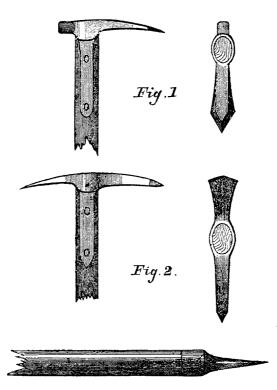
In the first place it is absolutely necessary that one of the cutters should be made in the form of a pick, as this is by far the best instrument for hacking into hard ice, and is also extremely convenient for holding on to a snow-slope, or hooking into crannies, or on to ledges of rock.
