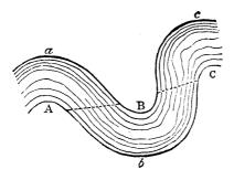
straight across, but follows the direction of a line connecting a promontory on one side to the nearest promontory on the other, as in the drawing; that is to say, from A to B, or from B to C, and *not* right across from B to *b*, from A to *a*, or from c to *c*. Along hollow
